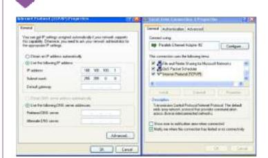
In order for the software to communicate with the camera, they must be on the same sub-network. All Phantom cameras have preset IP addresses on the same subnet — 100.100.x.x with subnet mask 255.255.0.0. It is customary to assign the controlling computer the IP address 100.100.100.1/255.255.0.0.
