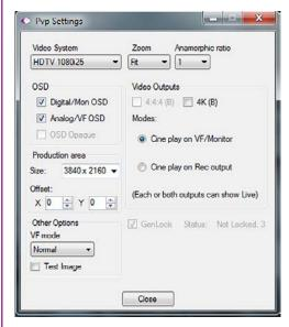
The camera's video mode and display settings are also set through PVP. Video systems will vary based on the country you are in, what kind of video monitor used, and the required display resolution. All available video setting for the connected camera can be found in the 'Settings' menu of PVP.
