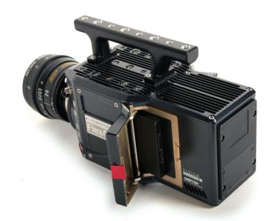
**Inserting a CineMag IV**
