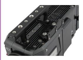
The adjustable arm mounts to the viewfinder, and then can be adjusted to the desired position on the camera body. An HD-SDI cable and 12V power cable are also included and connects to the front left side of the camera.
